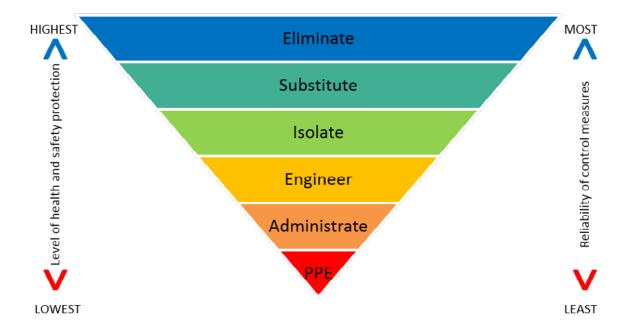
Applying the hierarchy of controls to COVID-19 may require multiple measures to be implemented in a workplace.
